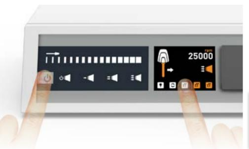
Press and hold "Start/Stop" and press the desired "Memory button" to save current burr speed, rotational direction and suction level.
