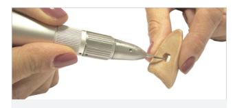
Final smoothing can be completed using a drill.
